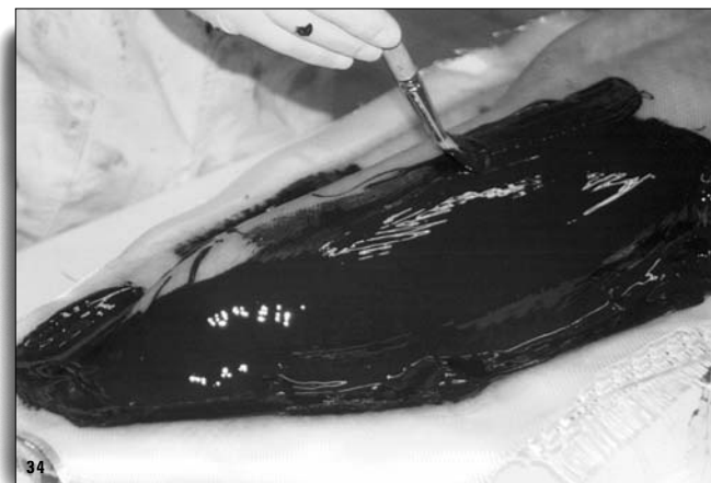
Finally, a 163 g/m 2 glass fabric is again laminated, to which the last layer of mould resin is applied ( Fig. 34 ).
