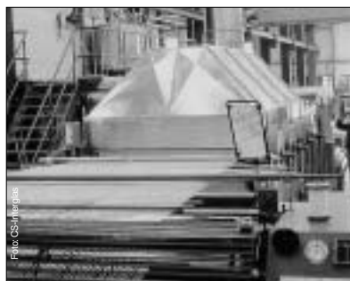
Schlichtemaschine zur Ketherstellung Sizing machine for manufacturing warps
