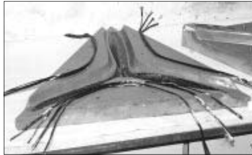
Prepared carbon rovings before impregnation and lay-up in the mould
