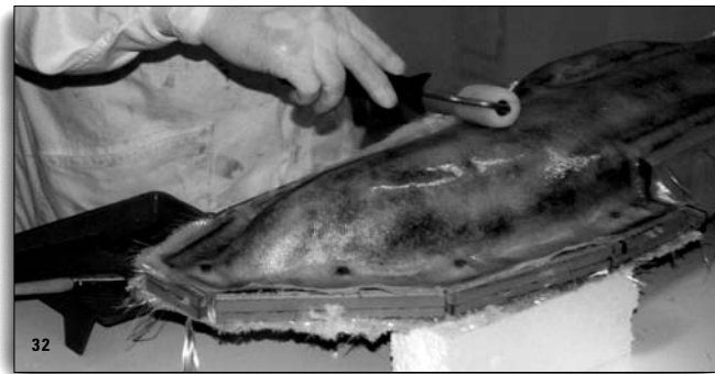
The first glass fabric layer 163 g/m 2 being laminated on top ( Fig. 32 ).
