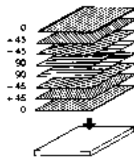
Multidirectionales (quasiisotropes) Laminat Multidirectional (quasi-isotropic) laminate
