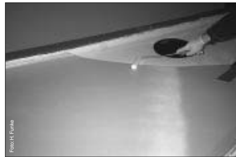
Aramidlaminat in der Tragfläche eines UL-Nurflüglers Aramid laminate in the structure of an ultralight flying wing
