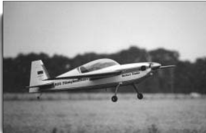
The F3A-X aerobatic model is built completely of honeycomb sandwich structures. The surface layers of 49 g/m 2 glass fabric and a 2 mm honeycomb core yield high rigidity with the minimum weight.
