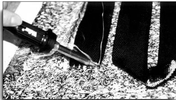
Soldering the connector sleeves on the carbon tape
