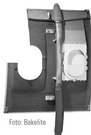
GRP honeycomb sandwiches as aircraft cowling segments
