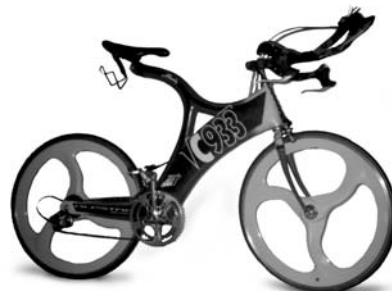
Triathlon bicycle of carbon-fibre reinforced epoxy resin (Karl Bodenhöfer, Waltenhofen)
