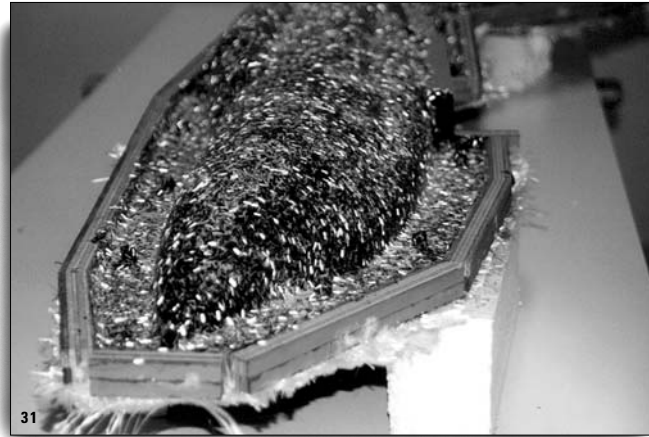
Chopped glass fibre being strewn in the "wet" overlay ( Fig. 31 ).
