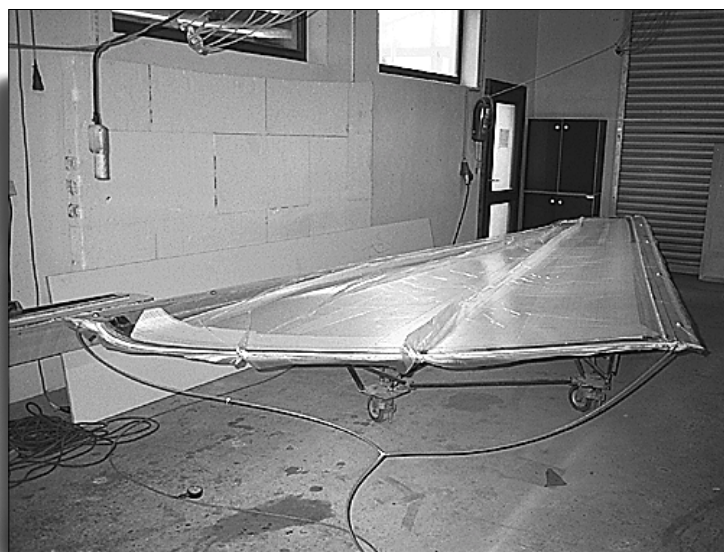
Vacuum-formed mould of an ultralight wing. The total pressure applied to the 9 m 2 mould is equivalent to 45 tonnes.
