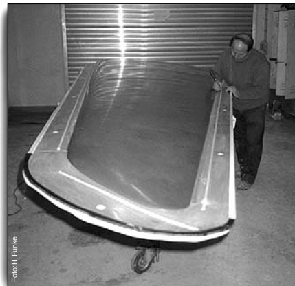
Master pattern prepared with release agent before the second half is demoulded.
