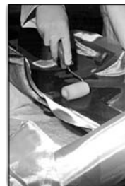
Herstellen eines Handlaminats mittels Schaumstoffwalze A hand lay-up laminate being made with a foam roller
