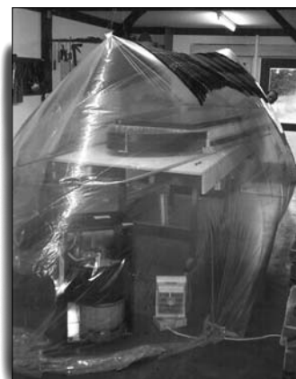
Hot curing in an annealing tent Important! For safety reasons, the annealing tent may not be left unattended when in operation!
